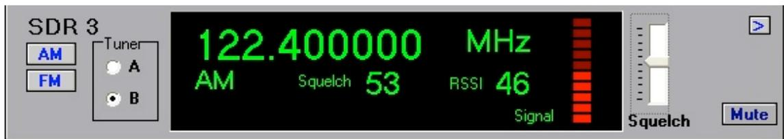
For each SDR channel there are buttons for selecting the tuner source, A or B. Then you can use the slider bar below to select the required frequency from the 8 MHz span of that tuner. The slider bar operates on the currently selected SDR channel - the one with the bright green display - the other three channels will have a darker green display. You can select a channel by clicking within the
